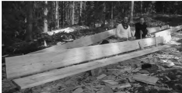
*Fig. 6 Boards, 6.2 metres long, resulting from a successful cleaving of one log into four boards. Photo Mattias Hallgren.*
