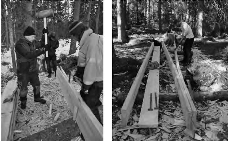
*Fig 1. Left; "Spårning" during the second cleaving of a boxed timber into boards. Photo Daniel Eriksson. Right; The second cleaving is almost done. Before the boards are separated so much waste material is hewn off as possible. Photo Karl-Magnus Melin.*
